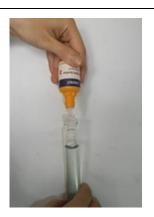
**3.** Wait 3 minutes. Add 7 drops of Reagent 3. White precipitate forms. Shake well until the precipitate completely dissolves.
