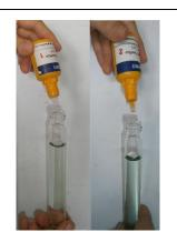
2. Add 7 drops of Reagent 1 and 7 drops of Reagent 2. Cap, then invert the tubes several times. Water turns light pink or light yellow, then light green or blue if sulfide is present.
