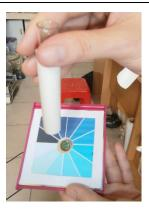
4. Place the tube into the comparator. Remove the cap. Hold the comparator with tube top pointing light source and tube bottom reflected in the mirror on the color chart.
